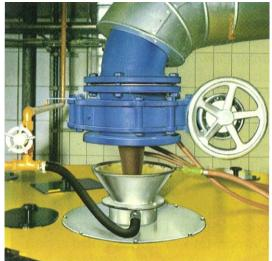
The flow into the centrifugal is controlled and regulated by an adjustable EGGER Iris Flow Control valve.
